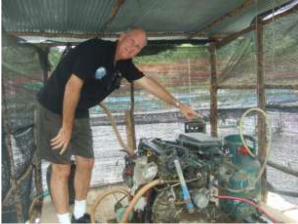
Truck engine running on cooking propane
